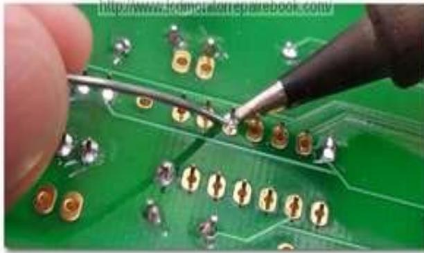
The second thing that I have seen people try to do is to use a soldering iron or soldering gun that does not have the screws holding the tip in place tightened tight enough. When you pull the trigger on a soldering gun, the tip should be smoking in 3 to 4 seconds. If it is not, tighten the screws that hold the tip in place. And I mean really tighten them TIGHT!!!
