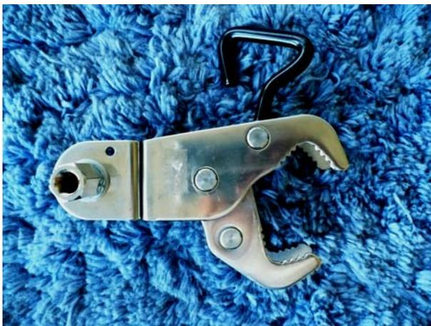
Don't forget you can mount a VHF or UHF antenna on this as well; it has a standard 3/8 x 24 mount on it but that can be replaced with the UHF mount or even an NMO adapter if need be.
