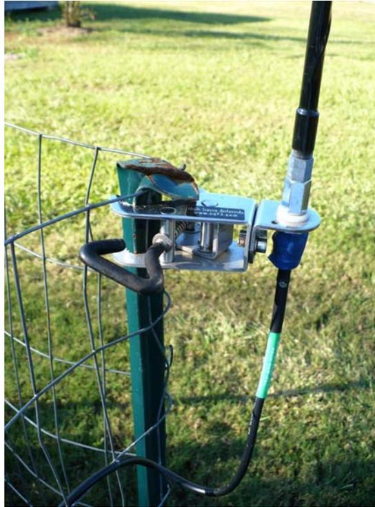
This type of mount, available from many hamfest and online vendors can be mounted on almost anything that will hold it. The jaws open wider than any other mount I've found. In this picture it is holding a Hamstick type antenna on a standard metal field fence post about 4 feet off the ground. The fence is serving as ground, like your metal car frame and skin would in a mobile situation. If all you have is a wood to mount the Jaws mount to it is easy to add some ground radials to the mount.
