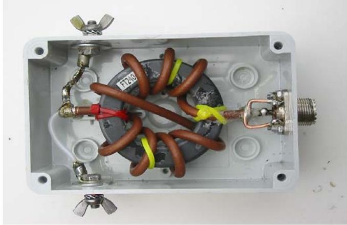
In its simplest form, the transformer type balun can be just some coax close wound around a four inch piece of PVC drain pipe. For a typical HF antenna 6 to 12 turns (more turns for lower frequencies) will work as a suitable impedance to keep the RF current from coming back down the shield. The ARRL Handbook and Antenna Handbook have examples of how to make one of these, and how many turns for what frequencies. These coax wound baluns are often called "ugly baluns"
